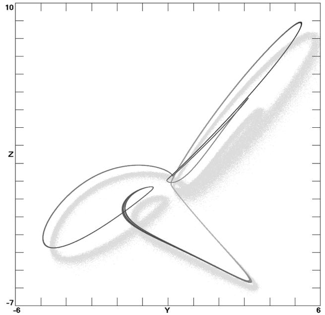
Fig. 5. A three-scroll chaotic attractor of system (16) with  $c_8 = 0.25$ .
