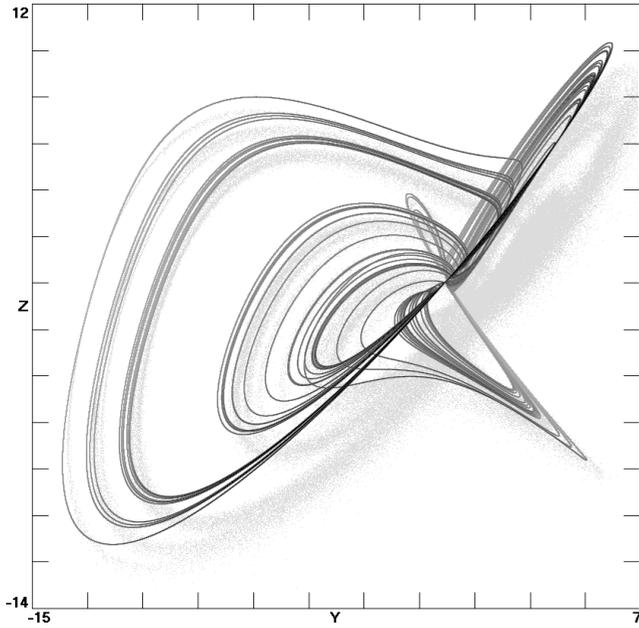
Fig. 1. A three-scroll chaotic attractor of system (16) with  $c_8 = 0.23$ .
