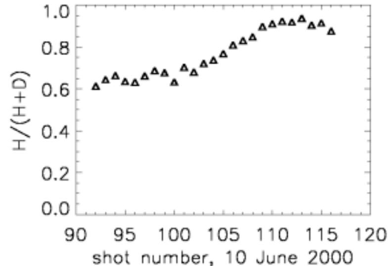
On 10 June 2000, deuterium discharges were run in the morning, and hydrogen discharges in the afternoon. The left-hand plot shows the RS spectrum from the first afternoon discharge (triangles). A two-parameter fit (solid line) gives the H and D concentrations ( $T_H$  and  $T_D$  are both assumed to be 200 eV). The right-hand plot shows the evolution of the fit H-to-D ratio during the afternoon.
