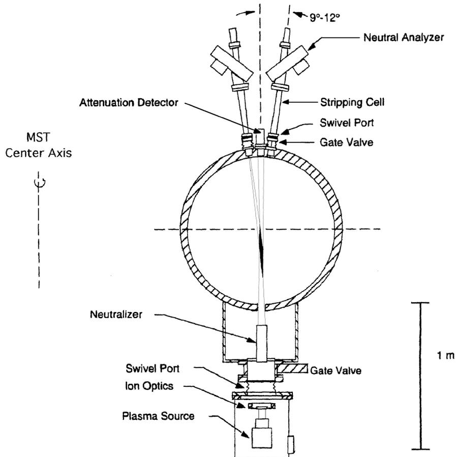
Small-angle scattering of beam atoms by plasma ions
