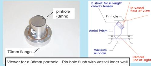
Viewer for a 38mm porthole. Pin hole flush with vessel inner wall.
