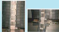
Inner wall portion of poloidal limiter:
