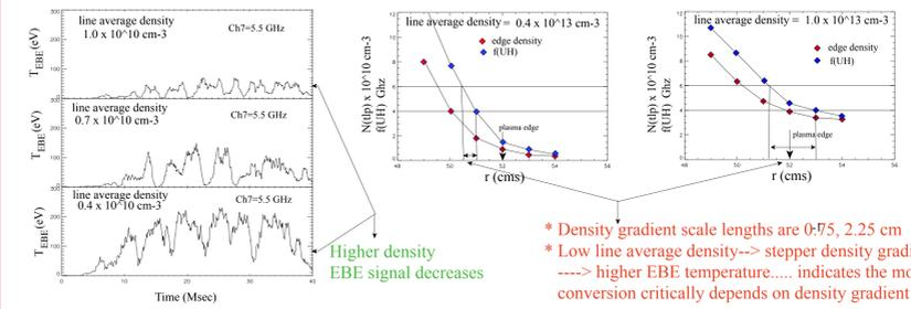
\* Density gradient scale lengths are 0-7.5, 2.25 cm
