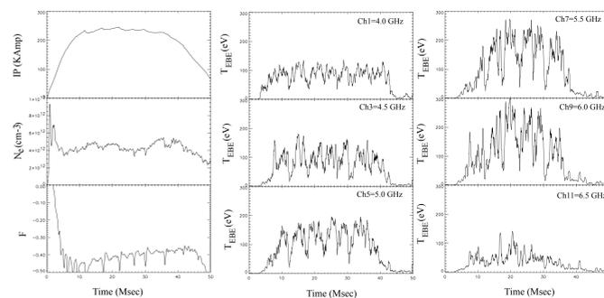
\* If radiation received assumed thermal, the radiation equivalent temp is close to plasma temperature
