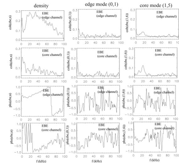
\* High coherence of ebe with n confirms the dependence of mode conversion on n.
