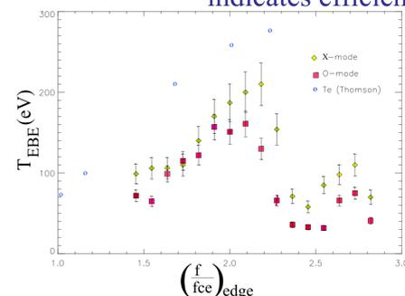
\*  $T_{(EBE)}$  for X-mode is higher than  $T_{(EBE)}$  for O-mode
