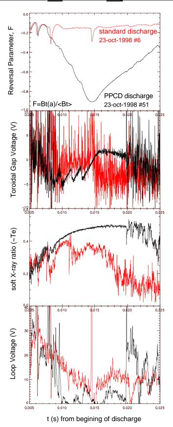
During a "normal" plasma discharge a series of 5 voltage pulses are applied to the MST shell to produce a magnetic field which is in the opposite sense to the established toroidal magnetic field, forcing flux out of the MST. This opposing B is thought to be due to a poloidally driven edge current.
