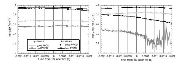
•The SXR ratio is proportional to temperature, for the most part, but is also sensitive to density and can be contaminated by line radiation. Furthermore, at these temperatures the SXR ratio is saturating in the nonlinear region of its sensitivity, and so may not be a good indication of the behavior of  $T_{e0}$ .
