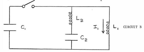
This circuit requires less capacitance in the parasite and doesn't require one to float  $C_2$  or  $L_1$ , but it does require a larger  $L_2$  and a higher voltage capacitor for  $C_2$  as shown in Table I.
