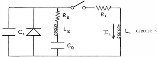
The addition of the diode across  $C_1$  has no effect on the preceeding calculations except to reduce the voltage reversal on the parasitic capacitor (see Table I). Voltage reversal of  $C_2$  can be eliminated entirely by providing it with its own crowbar diode, and there will be no effect on  $I_1$  since the voltage across  $C_2$  reverses after the voltage across  $C_1$  has been clamped to zero. The resulting waveforms are shown as dashed curves on figure 3.
