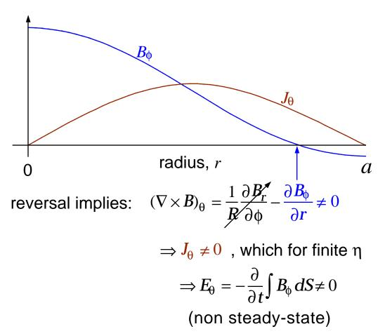
• But in an RFP, field reversal is maintained as long as toroidal current is sustained (  $\langle E_{\theta} \rangle = 0$  ):
